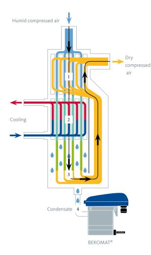
In the DRYPOINT® RAc, compressed air drying takes place via an optimum heat exchange through a counter-flow process over the cooling surface; the air flows constantly in a downward movement without turbulence.
